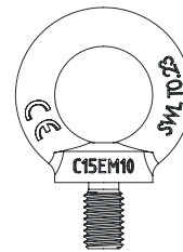
Fig. 3-1: Lifting eye bolts
